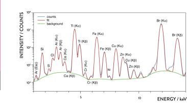
nanoXRF spectrum corresponding to the elemental maps (bottom left); monochromatic excitation at 17.5 keV and flux 10<sup>12</sup> photons/s
